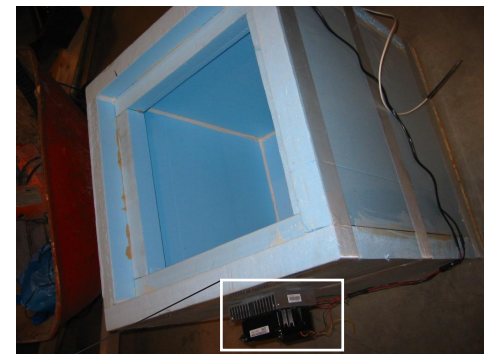
Dutch's Peltier cooled ferment chamber. Close-up of the Peltier Diode and muffin fan.
